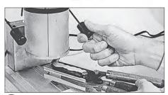
Fill mold through the sprue plate, puddle enough so all of the sprues are connected. Leave a ½1 to ½2 gap between the sprue plate and the nozzle when filling the mold cavities. NOTE Resting the sprue plate on the bottom pour spout while filling will pressure cast the cavities and may push molten material into the vent grooves, causing flashing on bullet.
