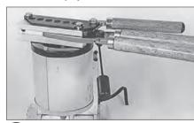
3 Pre-heat your mold by laying it on top of your lead melter or dip the corner of mold into molten metal for at least 30 seconds. If the lead sticks and solidifies on the mold block it's not hot enough.
