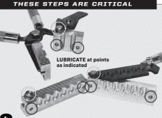
Lubricate your mold using beeswax or Permatex® anti-seize lubicant or equivalent. **DO NOT USE** Lee Liquid Alox as it will bake on the mold surface, preventing proper closure. **DO NOT USE** paraffin wax as it does not provide adequate high temperature lube and tends to migrate to the cavities, causing wrinkled bullets.
