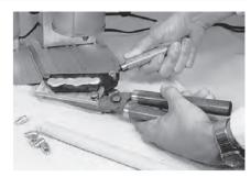
Immediately after sprue solidification operate the sprue lever if equipped or rap the sprue tang with a wood dowel. (A frosted surface will appear on the sprue puddle upon solidification).
