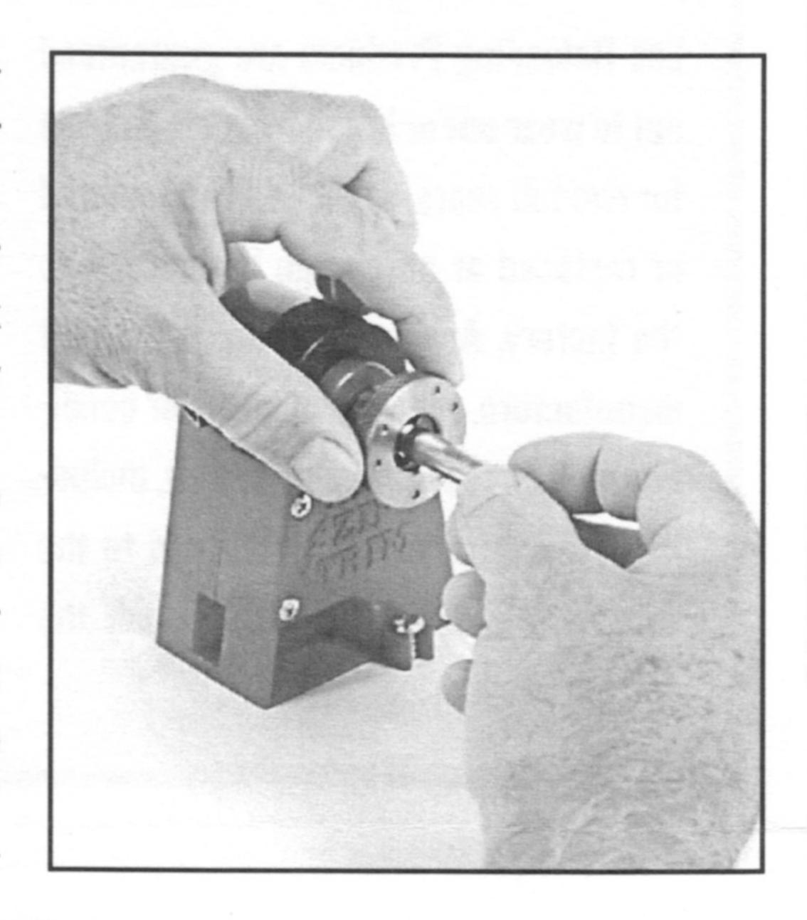
When changing cases, simply loosen the chuck from the tool about one half a turn, which should release the case allowing you to quickly replace it with another. When changing from cases with thin rims to thick, you may need to rotate the chuck body a full turn or more counter clockwise to accommodate the thicker rim.
