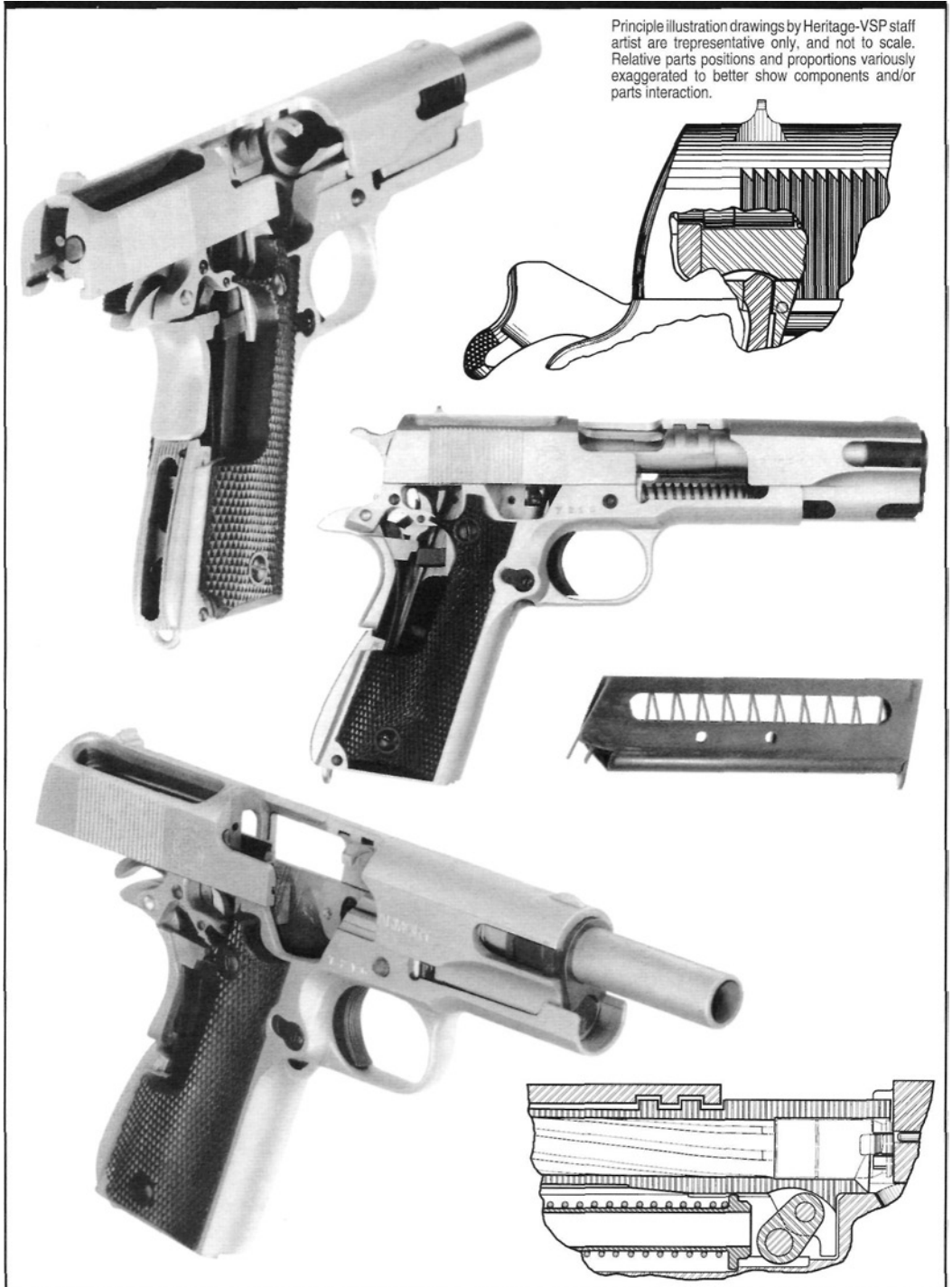
Figure 17- Cutaway pistols and partial sectional illustrations show M1911A1 interior views. Cutaway pistols are particularly useful in shop training and especially helpful in troubleshooting difficult problems. Virtually every parts function and interaction can be visually demonstrated in a cutaway M1911 pistol including: cartridge feeding; disconnect/reconnect function; hammer/sear engagement; trigger bow/disconnector/sear interaction; thumb safety/sear interaction; barrel link up/link down, and inertial firing pin function. Parts and interactions can be, freeze framed by simply stopping slide motion at any point. Headspace relationships also become apparent when headspace gauges are installed in cutaway barrels. Also see M1911/M1911A1 pistol basic function and cycle of operation beginning on page 37.
