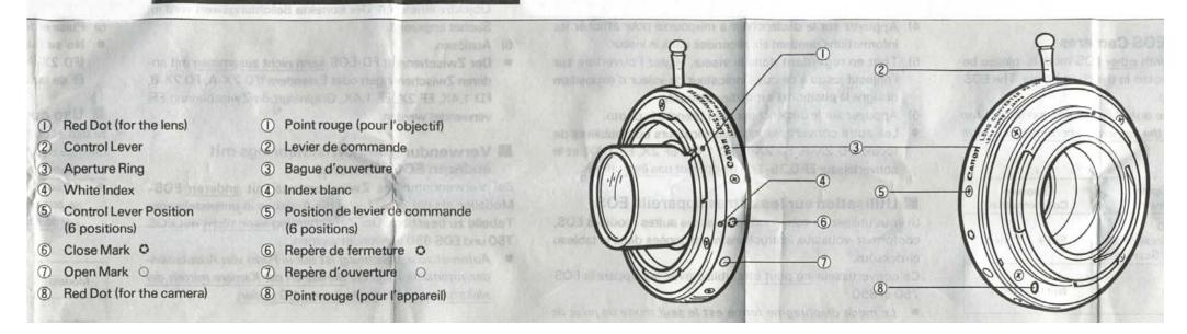
Thank you for purchasing the Canon Lens Converter FD-EOS. The Canon Lens Converter FD-EOS is an accessory exclusively designed to enable FD telephoto lenses to be used with the EOS-1. Despite the increase in the focal length by 1.26 ×, the shooting distance and optical performance remain unchanged.
