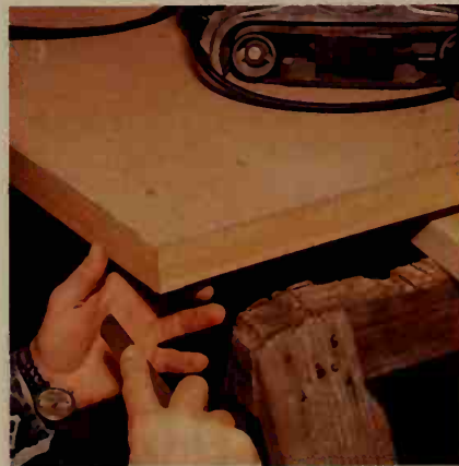
A file takes care of the finishing up. You can use the file for the entire edge if you do not have a router.
