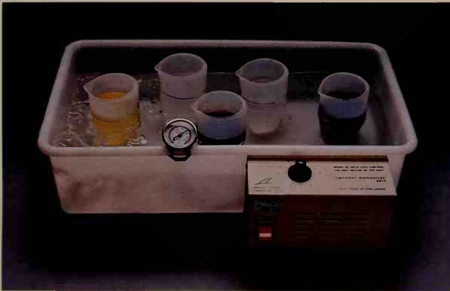
A temperature control bath with thermostatic sensor and a heating unit can ease the difficulties of maintaining solution temperatures.
