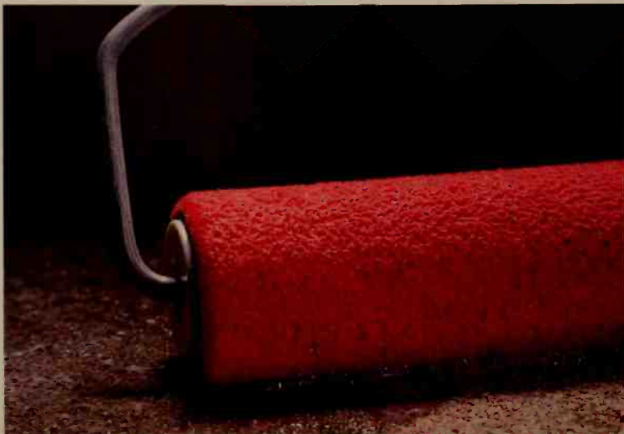
Dust is the enemy of good photographic quality. Limit the intrusion of dust by taping or caulking seams in paneling. Coat cement surfaces with a good sealer.
