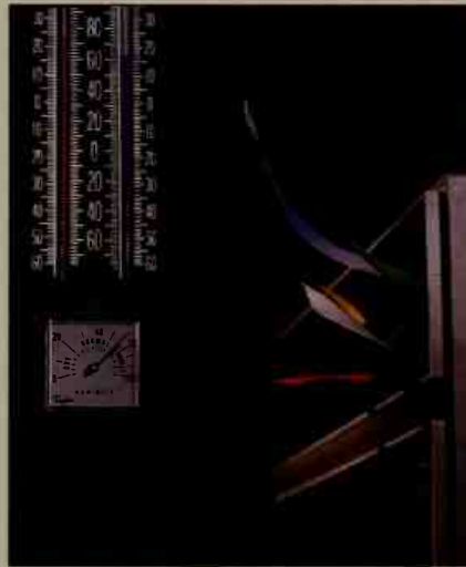
An air conditioner not only cools the room air but also extracts moisture from the air to provide some measure of humidity control as the wet bulb-dry bulb thermometer indicates.
