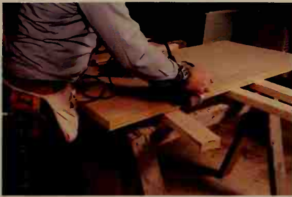
Preparing the top surface of the particle board with a sander is necessary to provide a better bond with the plastic laminate.
