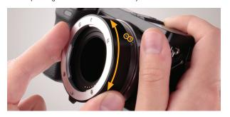
2. Line up the alignment marks on your lens and the tube.
